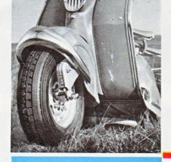
This fat and tough little fellow, together with his rear companion, has a fine tread which smooths the Prima driver's path and has a lot to do with the marvellous road-holding qualities of the machine. NSU continues to fit 8-inch wheels for a very good reason — they keep the centre of gravity of the vehicle low, and there are no weights high up which have to be balanced. The thick aircushion in the oversize low pressure tyres shows no tendency to bump even on the worst roads.
