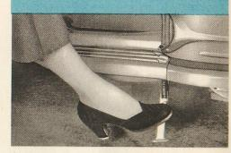
2 Choking. Pull the white button, - this automatically operates the choke control and also floods the carburettor. The Prima engine always starts immediately.
